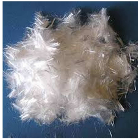
Fig. 1. Polypropylene Micro fibers used in CLC
