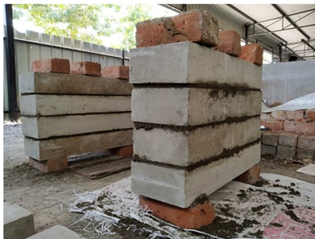
Fig.4. casting of CLC block stack bonded masonry prism
