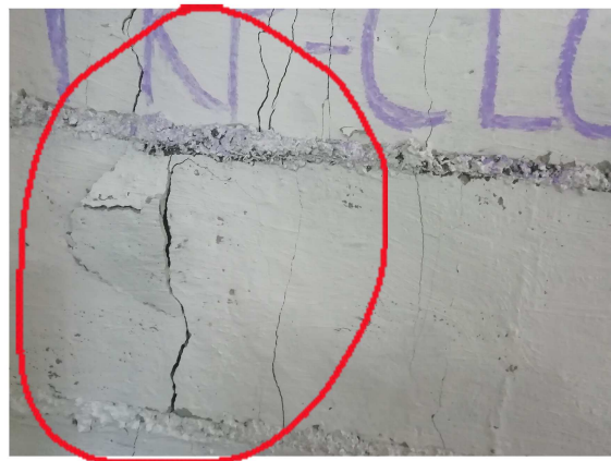
Fig.11. failure of mortar joint and micro cracks formation in fiber reinforced CLC prism
