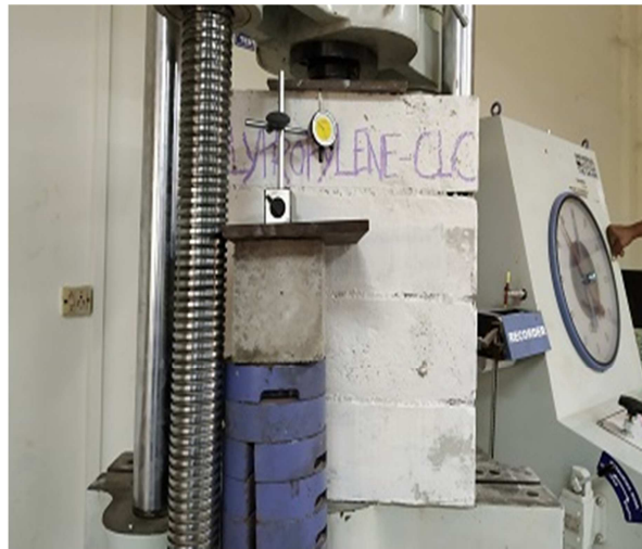
Fig.5. Testing of CLC prism
